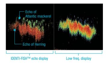
The following picture shows that the FSS-3BB is capable of identifying swim-bladderless fish. In this example, the Atlantic mackerel echo is displayed in light green.
